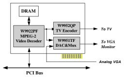
Figure-1 Application Example of W9922PF in Multimedia PCs through PCI
